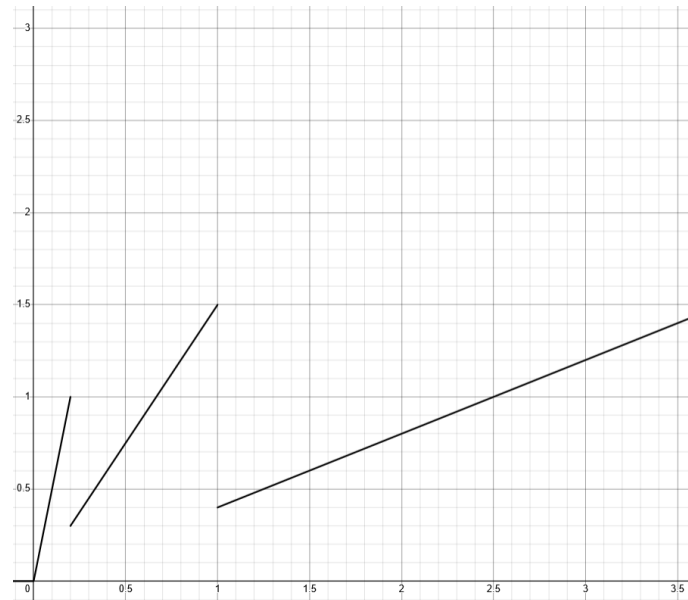
Figure 4.9: Piecewise linear transform with 3-sections. b_a = 0.2, b_b = 0.8, g_a = 5, g_b = 1.5, g_c = 0.4 . The transform is discontinuous due to absence of the adjustment term.
